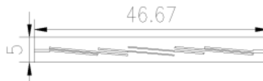
Fig.2 The designed parallel coupled filter.
